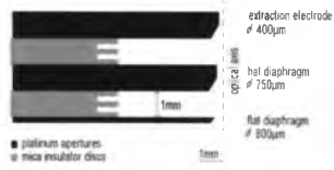
Fig. 2: Schematic view of the condenser lens
