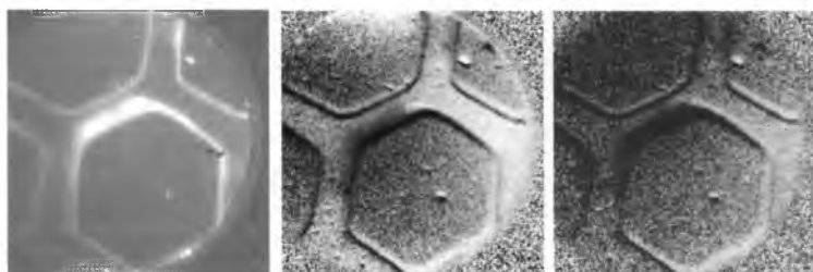
Figure 6: Lifetime contrast of hot electrons in a Ag microstructure (hexagons) on a gallium arsenide surface. Left: two-photon photoemission image without time delay, centre: pump-probe image with 60 fs delay ("lifetime image", single-pulse background subtracted), right: pump-probe image with 200 fs delay. FoV = 60 \mu\text{m} . (from [5])
