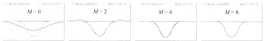
Figure 4: Fitting the axial function of Figure 1 using increasing numbers of Hermite basis functions.
