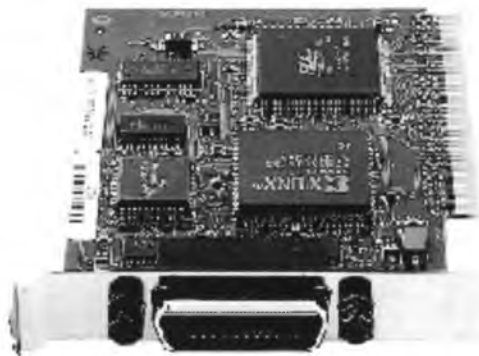
Figure 2: The Agilent 82350A PCI GPIB card having the IEEE-488 interface for accessing and controlling instruments and for data exchange.
