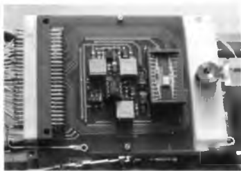
Figure 1: Experimental configuration of the detector in the microscope chamber (with the shielding removed).
