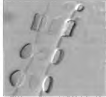
Figure 2: Geometry of the magnetic strip-line sample (left) and difference image of two PEEM images, one obtained in the static case (small constant field applied) and the other one with magnetic field pulses being applied at a rate of 1 \text{ MHz} (right).
