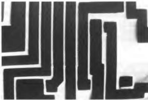
Fig. 2. Image of the positive resist pattern on Al surface. PE landing energy 620eV
